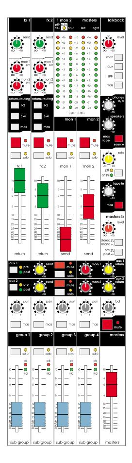
Both headphone outputs are controlled via the phones a/b rotary control, which provides a further 10dB of extra gain, as well as the output for control room speakers. In the same section, the source switch controls whether the tape or the master signal is present at the headphones and control room speakers if no solo button is engaged.
